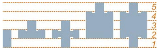
Figure 14: Diagram of variously proportioned base joints.
